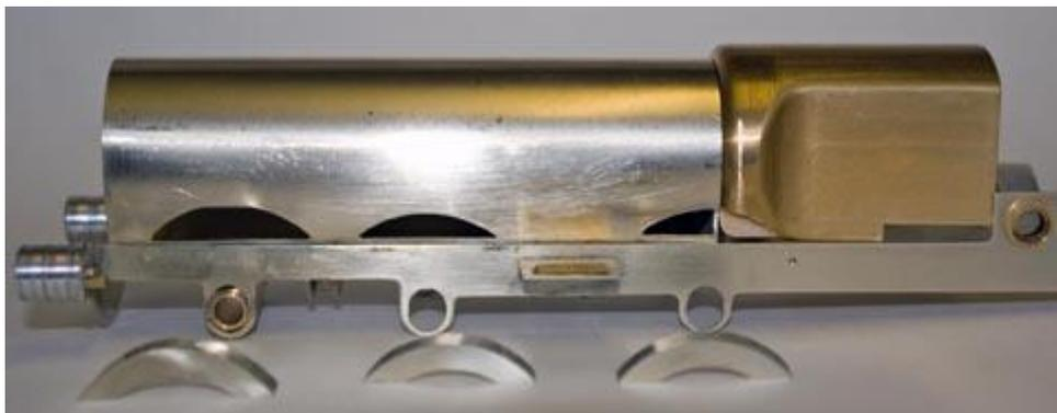
*Boiler and firebox mounted on inner frames, with splashers ready for assembly*
