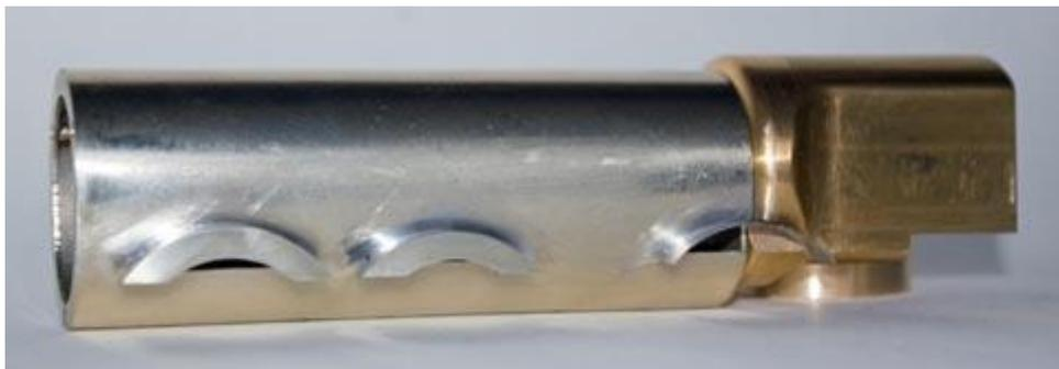
*Splashers soldered in place. The rearmost splashers had to be reduced in width because there is so little clearance behind the slidebars, and in doing so lost its front, but where it is, it is hardly noticeable*
