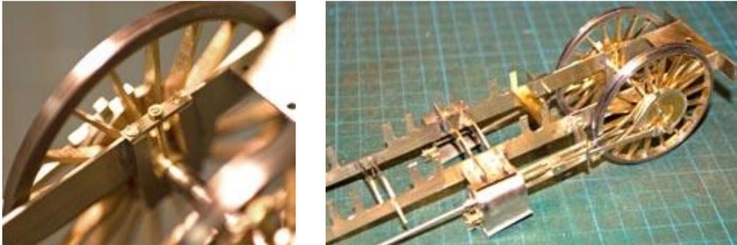
The right photo shows the majority of the inner frame assembly, upside-down. The change here has been to extend the stretchers supporting the boiler outside the frames in order to mount the cylinders, rather than putting the cylinders on separate extensions as before. The frames were slotted where the stretchers intersect them, using a slitting saw of the appropriate width, and when soldered up, the whole assembly is very rigid.
