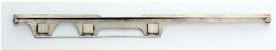
The outer frames are 0.4 mm nickel silver, also done on the pantograph mill. The step that runs along the outside is soldered along its length, and that also has the effect of keeping them straight. The rivets were done with my rivet press, and the various holes you can see are for the bolts used on the prototype. These will be represented using plastic mouldings from [Grandt Line](#) – I don't do absolutely everything myself.
