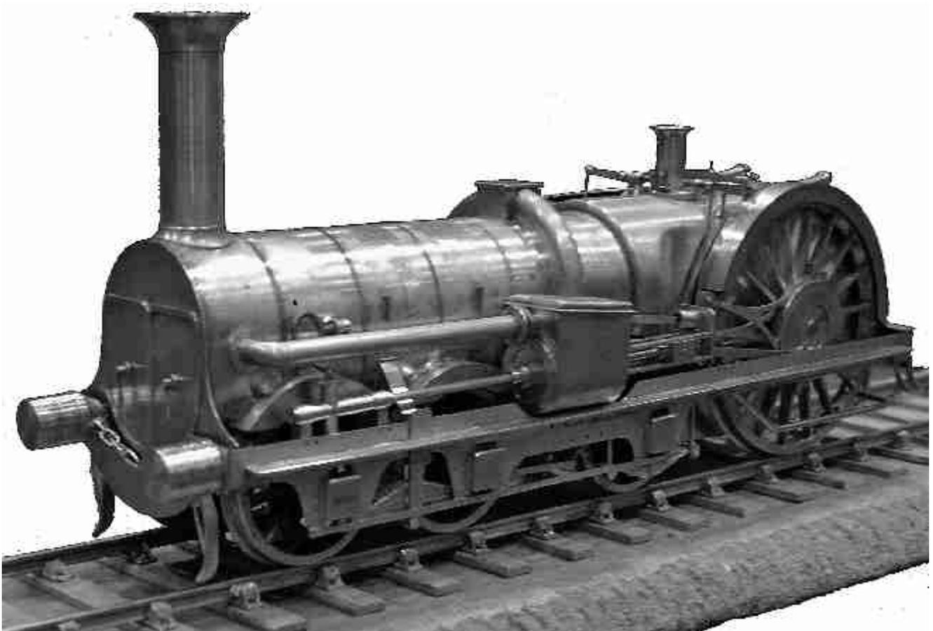
species of thermic siphon, the last of these dating almost a century before Mr Bulleid fitted them to his Pacifics! The firebox too was an odd shape, waisted to fit between the driving wheels, then expanding at the front end where it met the boiler.
