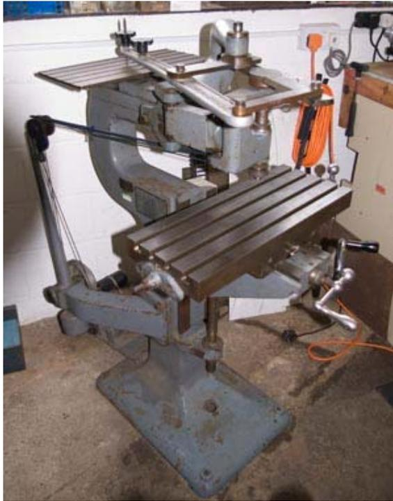
*The pantograph milling machine.*
