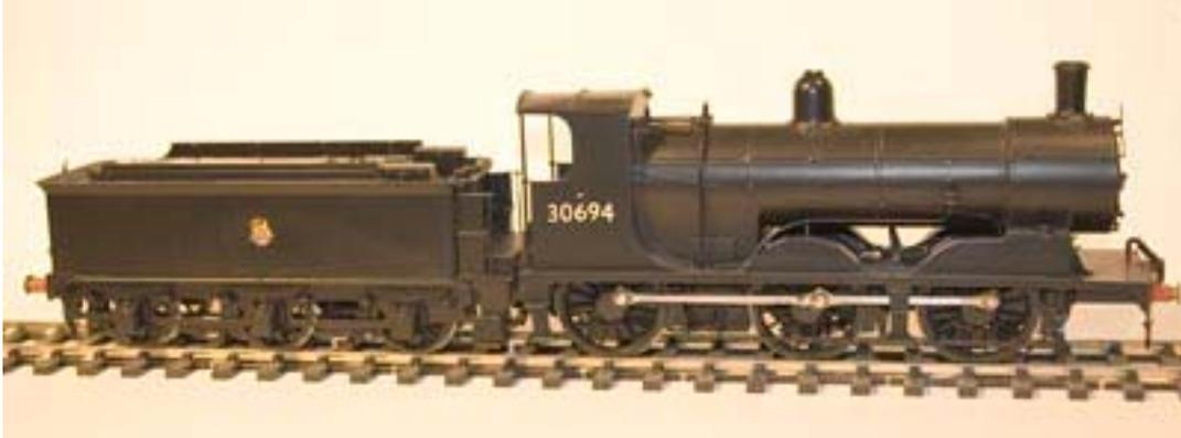
*The 700 class was one of my earlier models, but I still managed to include the connecting rods, crossheads, slidebars, and working inside valve gear. Detail like that, which is quite visible under the high-pitched boiler, is a must for me. The wheels are Slater's, but I had to modify them because the crank throw on this loco is unusually small.*
