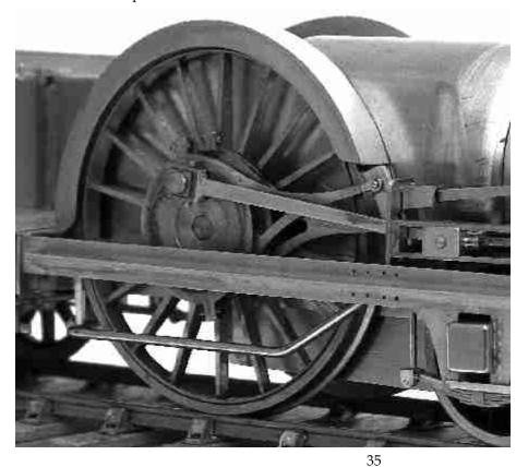
correctly. The driving wheels themselves, eight feet in diameter, are striking and there is an odd collection of leading and carrying wheels. The two front axles have wheels of different diameter and the centre wheels are flangeless.
